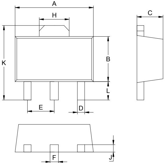
The diagram shows the top view and side view of a 3-pin SOT89 package. The top view indicates dimensions A (width), B (height), C (lead thickness), D (lead spacing), E (pin width), F (pin thickness), H (lead height), J (lead pitch), and K (total length). The side view shows the profile with lead thickness C and lead height H.
